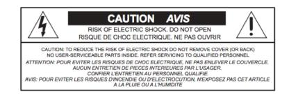
The Headphone Gizmo has an external power supply. Hazardous voltages are present within the supply and at the input of the Headphone Gizmo. Voltage may still be present on certain components even when the unit is unplugged.
