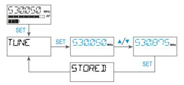
After switching the transmitter on, the standard display is shown on the display panel.
