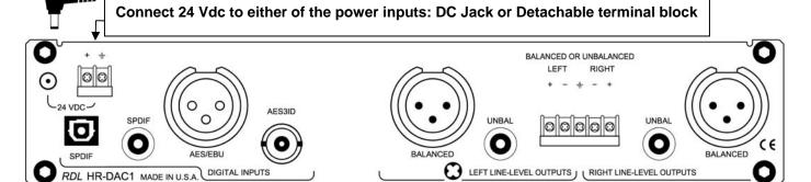
Connect one digital audio source to the appropriate input jack:
