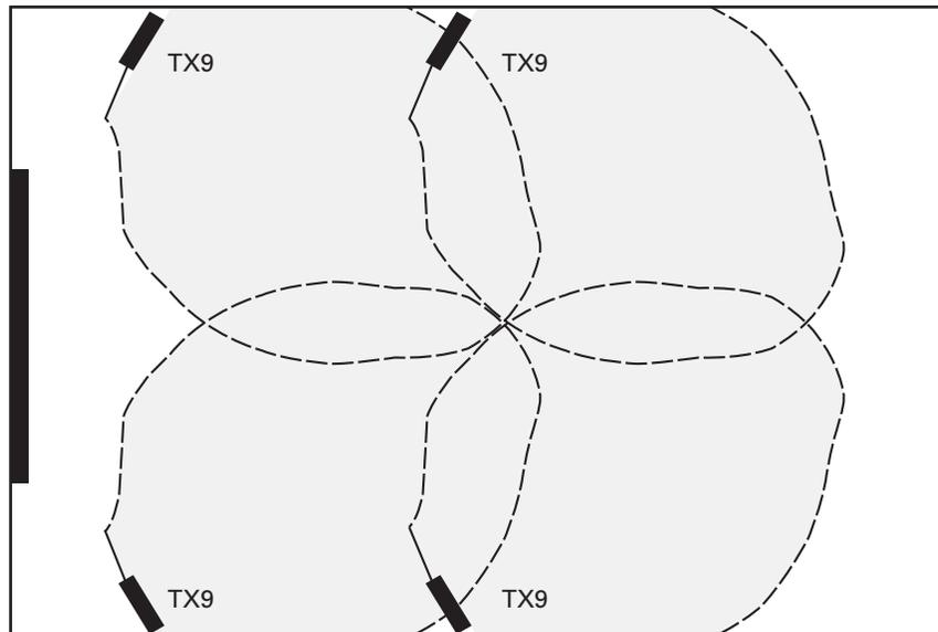
Fig. 8a above is a typical example of how multiple emitters are used to cover larger listening areas. Generally it is desirable for the illumination patterns to overlap. Note: The coverage area will vary depending on the infrared receiver being used; refer to Figures 4 and 7 to determine how many emitters are required to achieve full coverage of a listening area.
