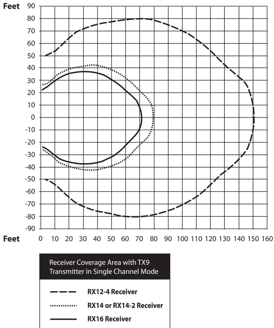
The coverage area for the TX9 will vary depending on the receiver being used. The diagram above demonstrates the receiver coverage when operating a single TX9 emitter in single channel mode. Patterns are direct radiation patterns.
