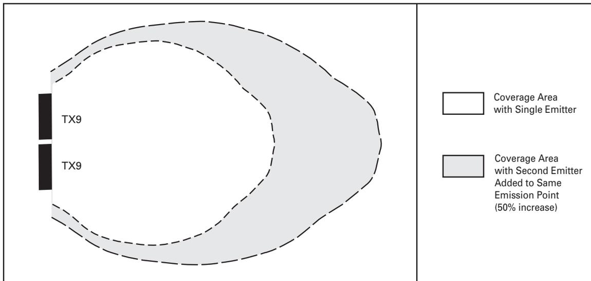
When two emitters are used at the same emission point in *single channel mode*, the overall coverage area increases 50%. When using an RX12-4 receiver, as a result, the coverage area will increase to an estimated 42,000 ft<sup>2</sup> (3,902 m<sup>2</sup>); the RX14-2 will increase to 5,250 ft<sup>2</sup> (488 m<sup>2</sup>); the RX16 will increase to 4,590 ft<sup>2</sup> (426 m<sup>2</sup>).
