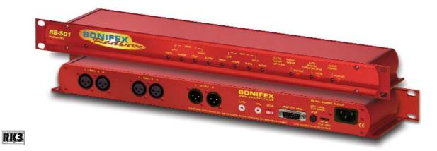
The RB-SD1 silence detection unit is a 1U rack-mount device used to monitor an unattended stereo studio feed and in the event of the signal going "quiet" after a given period the unit will switch through an alternative stereo audio signal. This signal could be a recorded message (e.g. "normal service will be resumed", etc), a feed from a CD player or minidisc machine, or an alternative recorded programme. Controls are provided to start external equipment and to provide remote status indication.
