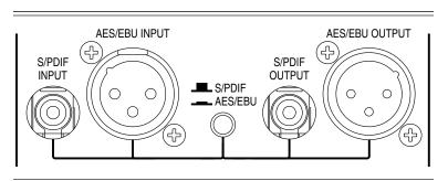
S/PDIF - AES/EBU SELECTION SWITCH - When the button is pressed in, the ADA1000 will process the information as AES/EBU format. When the button is released (the out position), the digital section will process the signal as S/PDIF information.
