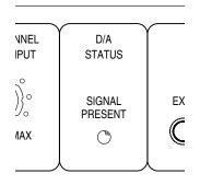
SIGNAL PRESENT LED - Lights to show that there is valid AES/EBU or S/PDIF format digital signal at the ADA1000's digital input port. This is especially useful to verify that the connections are correct when first hooking up the ADA1000 to a digital device. The ADA1000's D/A circuitry automatically locks to the sample rate of the incoming digital bit stream.
