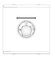
The ceiling speakers are secured by tightening the mounting screws from the front baffle. The ACS-40TS has three mounting screws, the ACS-55TS and ACS-55T have four. Tighten these clockwise, the swivel tables will rotate 90° and will then pull down onto the back of the tile to hold the speaker securely in place. A recommended torque setting of 0.5Nm and no more than 1Nm should be used to avoid over tightening.
