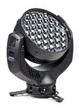
The impression X4 L features 37 RGBW LED's and offers full pixel mapping for ultimate graphical effects. But it doesn't stop there, as the X4 L also offers a super-fast 7:1 degree zoom from 7° to 50°; an indexing front accessory allowing for placement of beam shapers and similar options; smooth full range dimming with no color shift, all supported by the high output 15W LED sources that form the fixtures engine.
