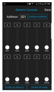
Once you have verified that the light fixture is responding to control signal from the app, tap the number field next to the word "Address". A new screen will pop up, prompting you to enter a DMX address. After you enter your desired DMX address, the app will return to the Generic Console screen. Finally, you must hit the ASSIGN ADDRESS button in order to save the new address into the fixture. Hitting the "Save" button will not save anything to the light fixture's memory.
