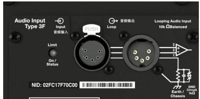
Figure 8: XLR 5-Pin Audio Connectors, Input and Loop Output
