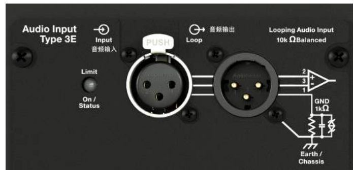
Figure 9: XLR 3-Pin Audio Connectors, Input and Loop Output
