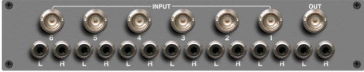
The **OMX-PSW6** is a high quality Video and Stereo Audio Passive Switcher. This device is designed as a general purpose signal switcher, or to fit the needs of facilities where "signal sniffing" is needed.
