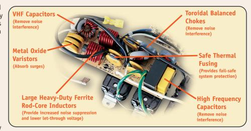
In addition, the Isobar, unlike other surge suppressors, provides more suppression components throughout the unit as *additional* lines of defense. The final safety measure is
