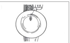
A more mellow sound is achieved by placing and ISOMAX 2 Omni microphone 2-3 inches down inside the bell using double-sided tape. Experiment with the face side down or up (do not cover the screen).
