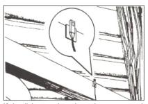
If the lid must be closed or removed, place an ISOMAX 2 Omni on one of the support braces near the middle of the instrument, as shown. Experiment with placement to avoid resonances. For stereo try one on the long support near the middle and one near the upper treble section.
