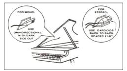
For mono: use double-sided foam tape to attach an ISOMAX 2 Omni facing the lid of the grand piano near the center board, or positioned over the strings on a mic stand. For stereo: place two ISOMAX 2 Cardioid mics on edge 1/8" apart facing left and right. The lid should always be open 3" to 6" (Closing the lid creates a "boxy" sound.)
