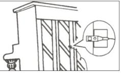
For upright pianos try affixing an ISOMAX 2 Omni to one of the central backposts, as shown. Experiment with placement as not all parts of the soundboard resonate the same. Two mikes in different areas should yield even better results.
