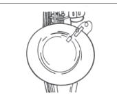
The ISOMAX 2 standard clip also works well when mounted at the top of the bell with the microphone positioned down, pointing inward.
