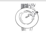
The Countryman Sax clip has foamcovered jaws that tightly grip the bell, with a stiff but adjustable wire that can be positioned at the center of the bell or twisted at the screw to capture sound through the keys.
