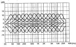
• Frequency Response (ex. All slider is set at a max. or min. position)
