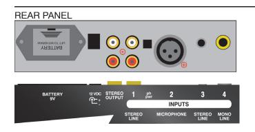
BATTERY 9V: Compartment for housing the 9V alkaline battery. DC POWER INPUT: Connects to the Rolls PS27; 12 - 16 VDC 150 mA power supply. The inside of the jack (the post) is negative, the outside is positive. <u>STEREO OUT</u>: Stereo RCA jacks with the main mixed signal at line level. <u>STEREO LINE (Ch 1)</u>: Stereo RCA jacks for connection to a line-level source such as a CD, cassette or video player.
