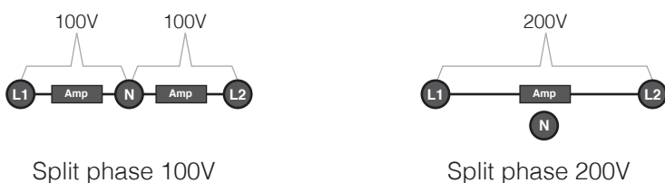
Figure 6:5: Two phase split-phase configuration
