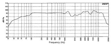
8CXT60 Frequency Response Measured in Q408 Enclosure
