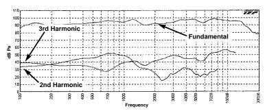
Fundamental vs. 2nd & 3rd Harmonics Measured in Q408 Enclosure (Transformer Bypassed)
