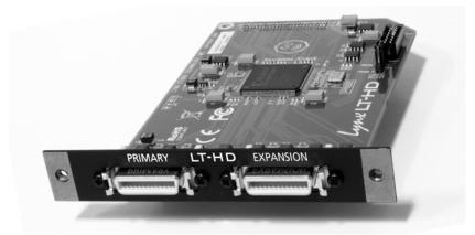
The physical connection between the Aurora/LT-HD and Digidesign Core, Process or Accel cards is very straightforward. Please note: we suggest only using DigiLink interconnect cables of 18" or shorter for optimal performance.
