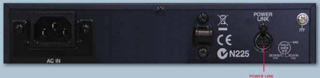
When running two S-OPT units in redundant mode, connect together via this power link to ensure backup power. If one power supply fails, the power link will share power with the second unit.
