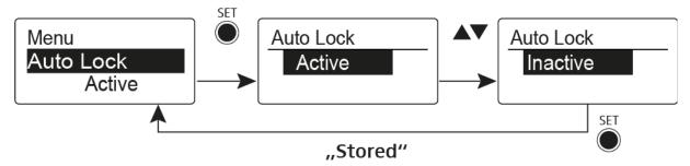
This lock prevents the wireless microphone from being unintentionally switched off and also prevents any unintentional changes to the transmitter's configuration. In the current standard display, the lock icon shows whether the lock-off function is currently switched on.
