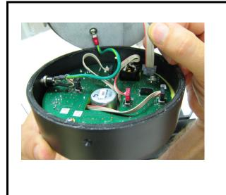
FIGURE 6. Connecting customer and operator assemblies prior to final mounting.
