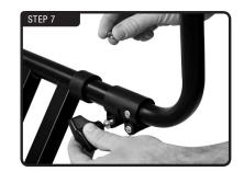
Install hand z-knob, washer, and hex nut. It is important to place the hand knob on the inside or stand will not fold fully. Also, be careful not to over-tighten the hand knobs because over-tightening may case cracking of the collar.
