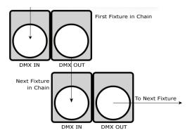
A quick note: Often, the setup for Master-Slave and Standalone operation requires that the first fixture in the chain be initialized for this purpose via either settings in the control panel or DIP-switches. Secondarily, the fixtures that follow may also require a slave setting.
