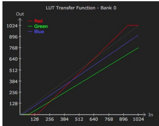
Figure 35. Example LUT Transfer Function Curves
