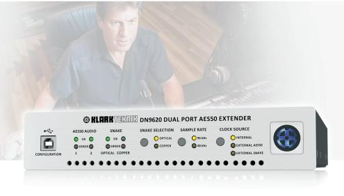
The DN9620 provides a high channel count solution to the 100 metre limitation that Ethernet and CAT5 cabling imposes on the physical size of AES50 networks. A pair of DN9620 units allow up to two AES50 connections (48 or 96 bidirectional channels channels at 96 kHz or 48 kHz sample rates respectively) to be extended by up to 500 metres via multimode optical fibre or 100 metres
