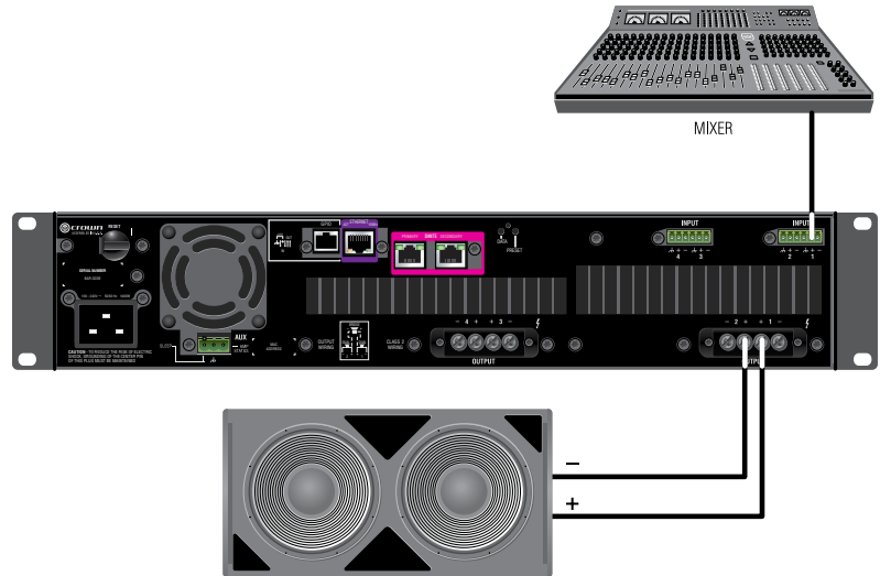
Figure 23: System wiring in Bridge Mono mode
