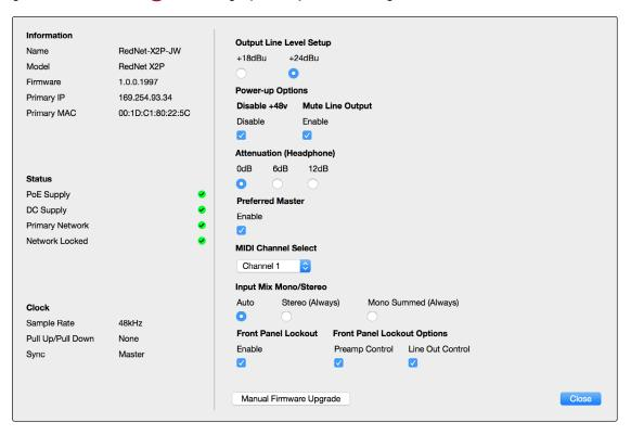
Output Line Level Setup - Sets the analogue Line output level at 0dBFS:
