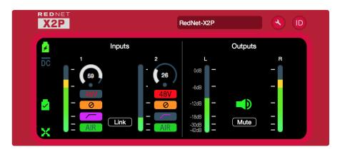
The image shows the input preamp channels' gain and function settings, level meters for inputs and outputs plus the power and network status indicators. Please refer to the section 'Device Control' in the RedNet Control Operator's Manual for full details of operation and setup using the software.
