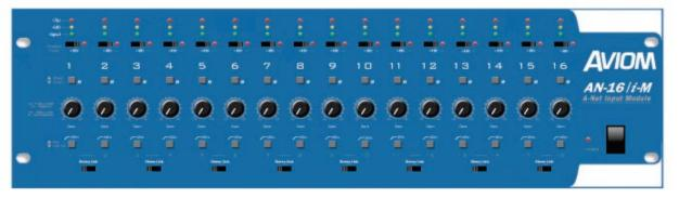
The AN-16/i-M Input Module allows microphone level signals to be used with AN-Series Distributed Audio Network products to create digital snakes and with the Personal Monitor Mixing System. The AN-16/i-M is designed to complement the existing products in the Distributed Audio Network line such as the AN-16/i Input Module and AN-16/o Output Module.
