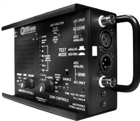
The Whirlwind Qbox-aes is a multipurpose testing device for troubleshooting digital AES-3, S/PDIF and analog audio signals. It is composed of two sections; a Send section and a Receive/Monitor section. A Test Mode switch selects Analog or AES testing operation. Audio is decoded and output through the built-in speaker or the 3.5mm jack. Test signals can be generated from multiple sources. In Line monitoring of an AES data stream is also possible with no alteration of the signal passing through.
