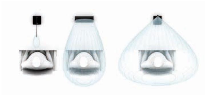
Recording area of a gooseneck microphone compared to a horizontal and vertical array microphone.
