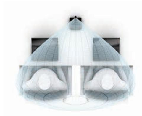
Due to the wide voice pickup two people can share one microphone. The microphone can also be used for video conferencing with several people. Due to the lateral placement of the microphone the workplace is free for laptops.
