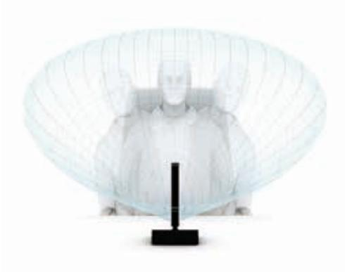
The vertical arrangement of the microphone array results in a horizontal corridor characteristic allowing maximum freedom of movement to the right and left without large volume fluctuations. The attenuation above and below the microphone limits the recording of signals and noises from the ceiling and table.
