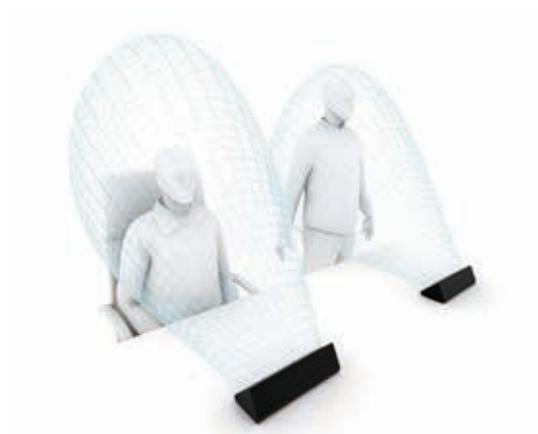
The horizontal arrangement of the microphone array results in a vertical corridor characteristic, which allows enhanced freedom of movement. Whether the speaker is sitting or standing, the volume and audio quality always remain the same. People on the left and right from the speaker are faded out.
