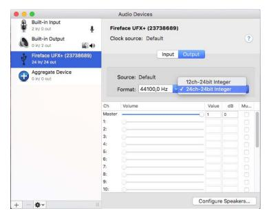
Mac OS X supports USB Audio 2.0, even with more than 2 channels. The UFX II offers 24 input and 24 output channels at up to 96 kHz. It is shown as "Fireface UFX II (xxxxxxxx)" in the Audio MIDI Setup, in both normal and CC mode. In CC mode the USB Settings will vanish from the Dock, and TotalMix will – if at all – show a 'disconnected' UFX II.
