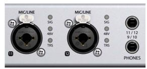
The analog outputs 9 to 12 feed the headphones outputs **Phones 1** and **Phones 2**. These low impedance outputs of highest quality are able to drive headphones at higher levels undistorted, no matter if low or high impedance headphones are used.
