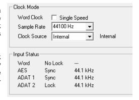
This way, configuring any suitable audio application for digital recording is simple. After selecting the correct input, Fireface UFX II displays the current sample frequency. This parameter can then be changed in the application's audio attributes (or similar) dialog.
