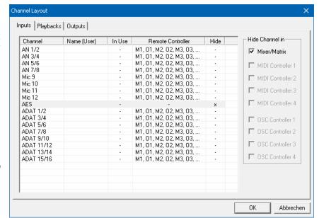
In the above example the AES input channel has been made invisible. When AES is not used this is an easy way to remove it from the mixer completely. A more complex setup would be to only show all channels of the drum section, the horn section or the violins.
