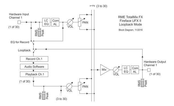
The block diagram also shows why with activated Loopback the EQ of the Hardware Output is now within the record path. With Loopback active the EQ of the input is not in the record path, only in the monitoring path, even when the Option DSP - EQ + D for Record is activated.
