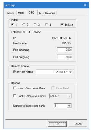
➤ Number of faders per bank. Available choices are 8 (default), 12, 16, and 24. Note that when working in underperforming networks, especially wireless, a higher number of faders might not work as smooth as expected.
