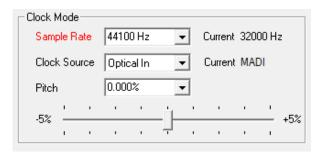
Under ASIO the audio software sets the sample rate, so that such an error will usually not happen – but it can too. In slave mode the external sample rate has priority. Feeding 44.1 kHz will prevent the ASIO software to set 48 kHz – obviously, as the only way to do so would be to enter a different clock mode (Master/Internal).
