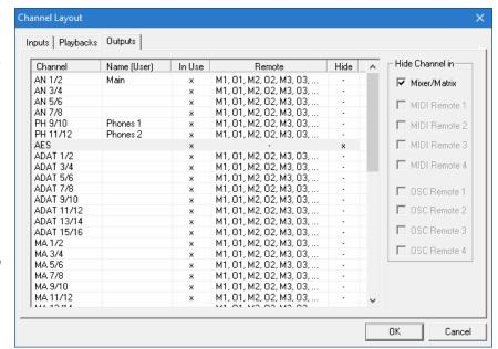
In the above example the AES input channel has been made invisible. When AES is not used this is an easy way to remove it from the mixer completely. A more complex setup would be to only show all channels of the drum section, the horn section or the violins.
