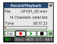
Playback mode turning encoder 2 allows to change the current playback position.
