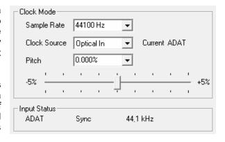
This way, configuring any suitable audio application for digital recording is simple. After selecting the correct input, Fireface UFX+ displays the current sample frequency. This parameter can then be changed in the application's audio attributes (or similar) dialog.
