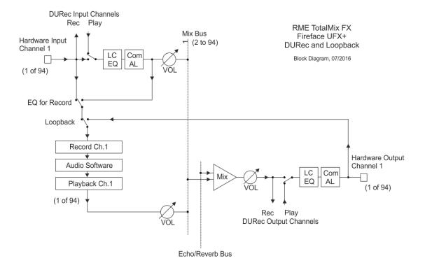
The block diagram shows the signal flow for various situations, depending on the state of *Loopback*, *EQ for Record* and *Play active*. In the diagram Loopback and EQ are switched to off, but a playback is active in the input.
