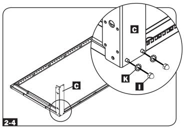
Fasten a top bracket II to the threaded M8 stud at the end of the assembled top section with an M8 acorn/cap nut II and M8 washer II. Tighten 90%. (The threaded M8 stud should pass through the vertical rail first, then the top bracket.)
