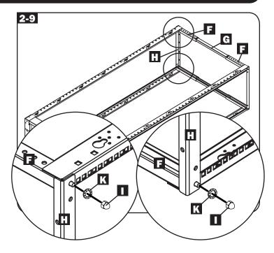
2-10 Place the rack upright on a level surface and confirm that the rack is stable. Tighten all nuts and bolts until fully secure. (If you are installing optional casters, follow the instructions in Section 3, then return to this step.)
