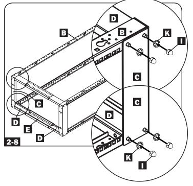
2-9 Fasten a top bracket II to the threaded M8 stud at the end of the assembled top section I/C / I with an M8 acorn/cap nut II and M8 washer II. Also fasten the base bracket to the threaded M8 stud at the end of the other assembled bottom section with an M8 acorn/cap nut II and M8 washer II. Tighten 90%. (The threaded M8 studs should pass through the vertical rails first, then the top bracket.)
