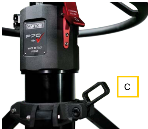
Figure 4 — Lever C to secure the column to the skid
