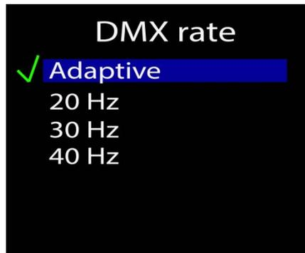
Select one of four options for **DMX out refresh rate:** Adaptive, 20Hz, 30Hz, 40Hz.
