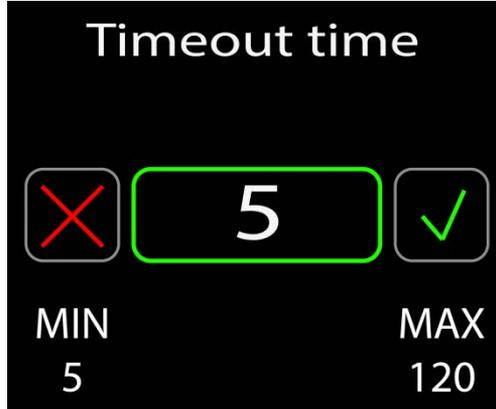
This setting determines how long the IQ Micro will wait before using the **Source Loss** setting. This time is set in seconds. (5-120). Once the source loss timeout threshold has been reached, the IQ Micro will revert to the Source Loss timeout setting.
