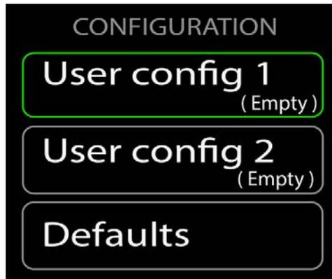
The configuration menu is used to save and load User Configurations, load system defaults, and reset system settings.
