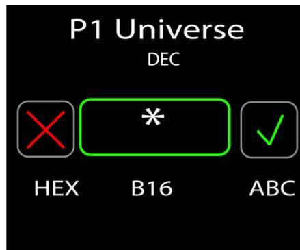
In this window, the universe number can be set (from 0 to 32767) for the selected DMX port (the example shows “Decimal” Universe Format).
