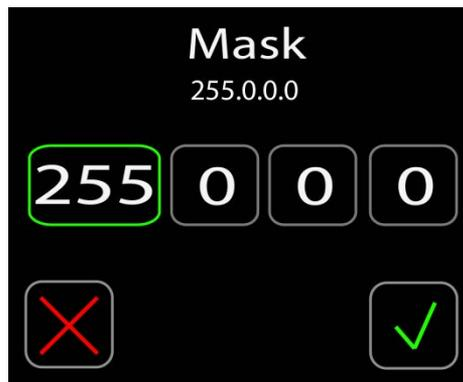
The Subnet mask of the IQ Micro can be changed. To change the assigned Subnet mask, replace the current network Subnet mask with the desired network Subnet mask.
