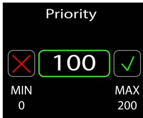
Here port priority (0 - 200) can be set. When signal is lost for the highest priority port, the DMX signal will be taken from the port that has the next highest priority when addressed to the same universe. This is useful when two DMX sources need to be prioritized while operating as the same DMX address. When two priority levels are the same, HTP Merging will occur.
