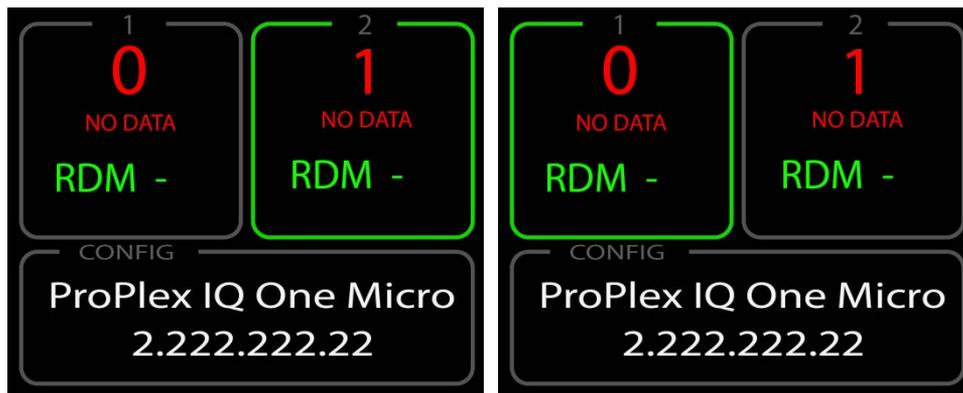
Using the <UP>, <DOWN>, <LEFT>, <RIGHT> buttons, select the DMX port to be changed. In the above images, the left image shows Port 2 selected and highlighted, and the right image shows Port 1 selected and highlighted.
