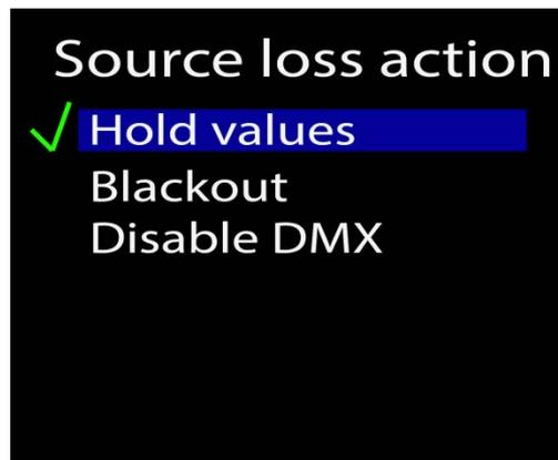
When the "**Hold values**" setting is selected after the DMX source is lost, the IQ Micro holds the last DMX values it received and continues to output these values until incoming DMX has been restored.
