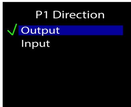
This setting is used to change the port direction from input to output.
