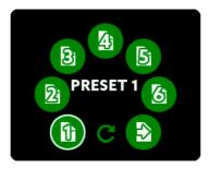
After selecting the number of the preset to load, you can choose which parts of the preset you want to load: Gains of the analog inputs and/or levels of the analog outputs and/or routing.
