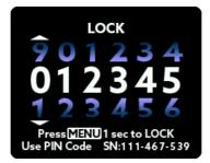
After entering the correct number, hold down the MENU button for a few seconds to activate the lock.
