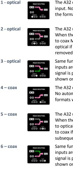
The A32 only uses the optical MADI input. No automatic switching between the formats will happen.
