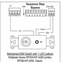
Alternate Sequence Mode (ASM) allows for the bypassing of selected outputs for partial system
