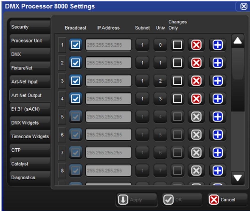
Figure 3.11. Art-Net Outputs pane of the DMX Processor Settings window
