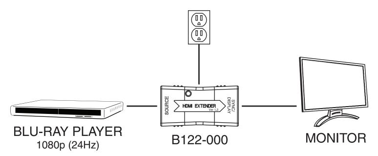
Connect the longer HDMI cable between the source and the connector on the B122-000 labeled "Source."
