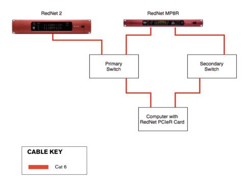
RedNet units with only one network port must be connected to the Primary Switch Only.
