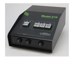
signals used to communicate with producers, directors, spotters, or other behind-the-scenes production personnel. A status LED is associated with each of the talkback pushbuttons. The pushbutton switches use gold-plated contacts for reliable longterm operation and include backlighting using white LEDs. Three rotary controls allow the user to adjust the content and level of the headphone output.
