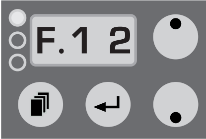
Adjusting of the fog time in seconds (1-99)
