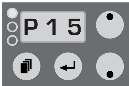
Adjusting of the output/pump in steps of 1% (1-99%)
