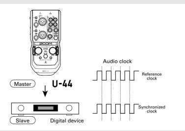
The  $\mathbf{U-44}$  is operating as the master, and the audio clock of the  $\mathbf{U-44}$  and the other digital device are synchronized.
