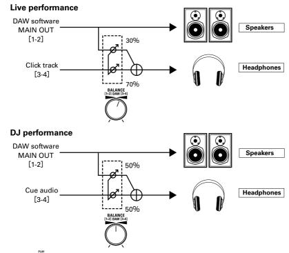
1. Turn to adjust the balance between computer playback signals 1-2 and 3-4.
