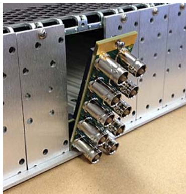
Figure 2. Rear Card Inserted Into Frame Seating Slot
