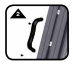
2. Position handle in place by lining up holes in handle and holes in handle mount.
