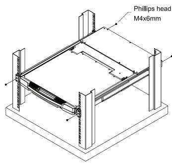
6. After determining that the RM-KB-LCD17KVMHD is lined up and operating correctly, finish by fully tightening the front attachment screws inserted in
