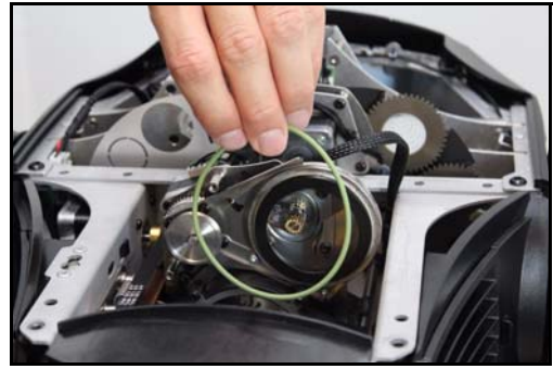
Figure 18: Removing the prism drivebelt
