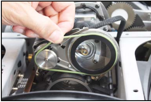
Figure 18: Removing the prism drivebelt
