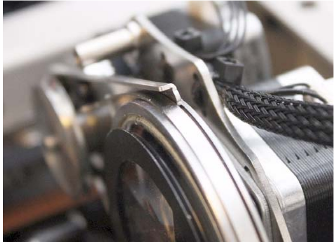
Figure 20: Correct prism location
