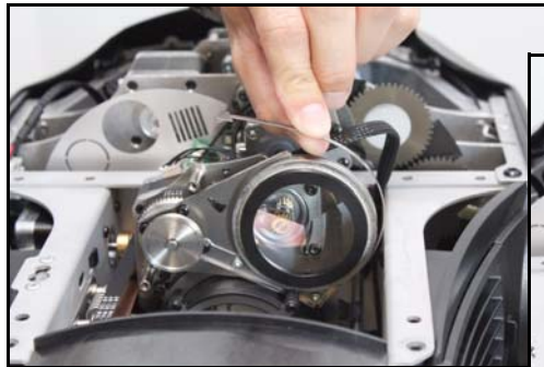
Figure 19: Removing the rotating prism
