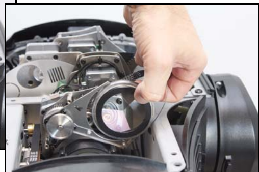
Figure 19: Removing the rotating prism
