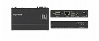
The **TP-125xl** is an extended range twisted pair transmitter for computer graphics video, unbalanced stereo audio and bidirectional RS-232 control command signals. It converts the input signals to a twisted pair signal and transmits them over CAT 5 cable to a compatible receiver.
