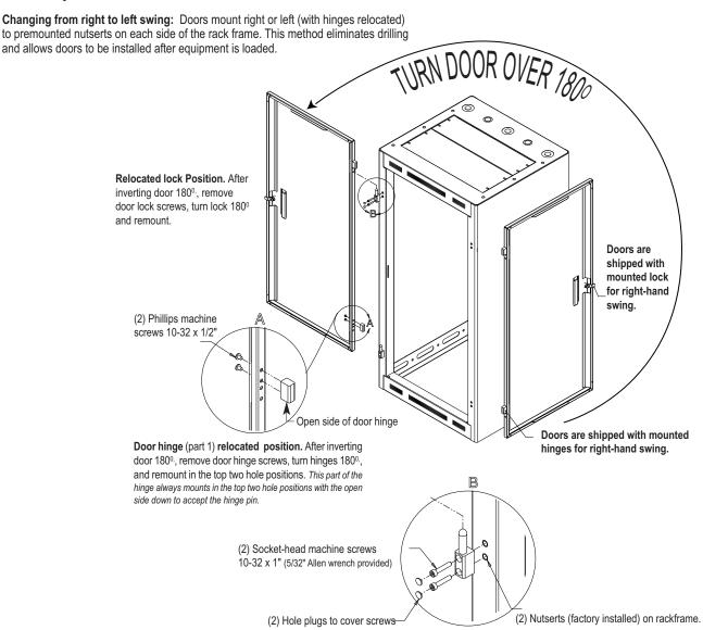
**Door hinge pin** (part 2) **mounts to cabinet without drilling.** The second part of the door hinge (pin) is always field installed to factory mounted nutserts. Nutserts are located on the front left and right of cabinet.
