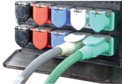
2. Insert the Cam connector into the receptacle and rotate Cam connector at least 90 clockwise degrees to lock
